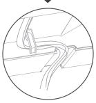
Hook the wire into the buckle and go down from the wire slot.
