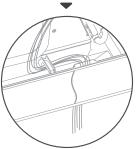
Replace foam gasket over wires.
