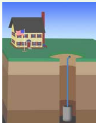
Ground Water: used when there is abundant well water; no piping for heat exchange fluid is required.
