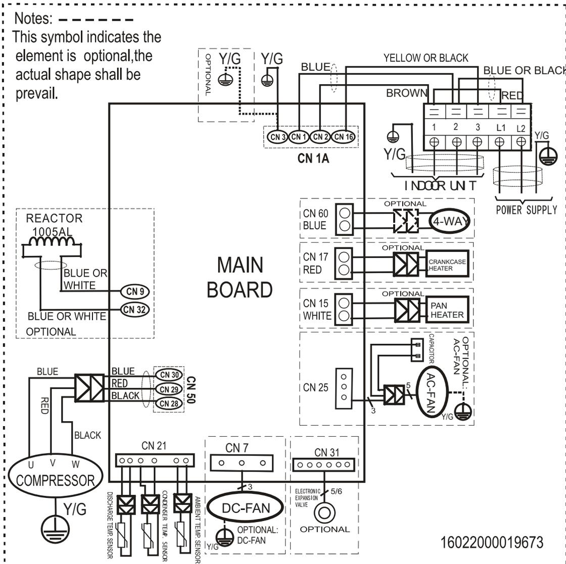
Outdoor unit wiring diagram: 16022000019694
