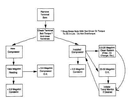
**Megohmeter Test Procedure**
