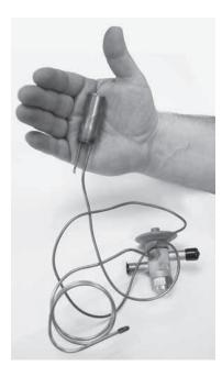
Suction pressure increases when warmed and decreases when bulb is cooled in cup of ice water
