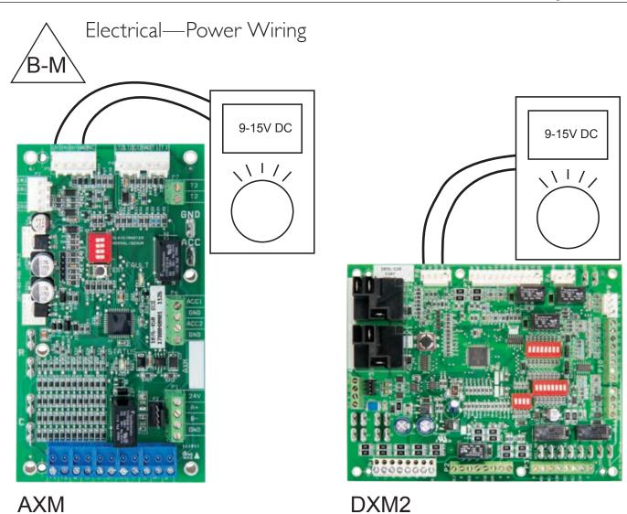
Note: Check the unit voltage with the harness connected and unit powered up.
