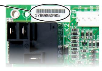
Note: Any board version lower than 3.3 should be replaced if experiencing any odd symptoms or lockouts that are unexplained
