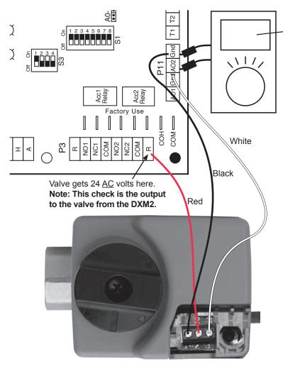
You should see 3.3-10 Volts A/C D/C when valve is functioning properly.
