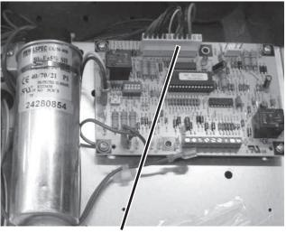
Remove this Molex plug to check resistance of the FP1/ LT1 sensor
