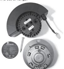
2) Remove plastic cover to remove Torx head screws.
