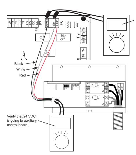
24 volts <u>DC</u> First stage auxiliary heat
