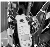
With the rectifier removed from the compressor, verify 15-27 VDC.
