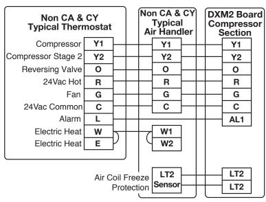
Note: LT2 sensor is shipped on HZ units
