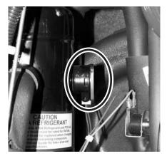
When rectifier is removed, verify that pins are not bent.
