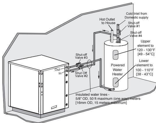
Figure 4: HWG Double Tank Installation
