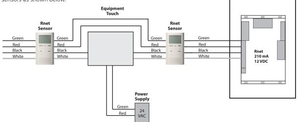
Note- The Equipment Touch does not require the user to set an address for it.
