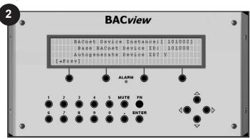
The device instance is typically six digits long. The last two digits correspond to the addressing rotary dials so these should not be changed using the BACview6.
