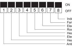
Indoor Fan Motor Rotation Speed Select Fan CYC. For Cooling Electric Memory Room Freeze Protection Heating priority(Only available for panel control) Electric Heat Heat Pump Anti-cold air
