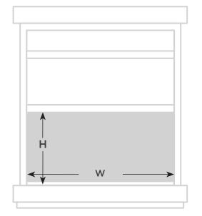
Your air conditioner is designed to install in a wooden sill double-hung window. All wood parts of window must be in good shape and able to firmly hold the needed screws. If not, make repairs before installing unit. If your storm window frame does not allow the clearance required, correct by adding a piece of wood, or by removing storm window while room air conditioner is being installed. The standard parts are for window dimensions listed below.
