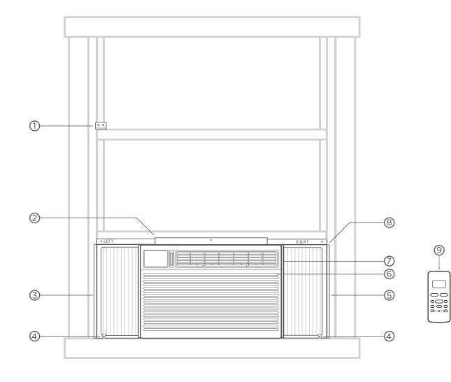
(1)Safety Lock and 5/8in Screws 2 Top Rail and 3/8in Screws Frame Assembly(Left) 3 (4) Safety Lock and 5/8in Screw Frame Assembly(Right) (5)Air Conditioner unit 6  $\bigcirc$ Side Retainer(both side) Window Sash Seal Foam (8) Remote controller  $(\mathfrak{G})$
