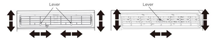
The louvers will allow you to direct the air flow Up or Down(on some models) and Left or Right throughout the room as needed. Pivot horizontal louvers until the desired Up/Down direction is obtained. Move the Lever(s) from side to side until the desired Left/Right direction is obtained.
