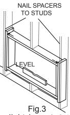
**NOTE:** If wall thickness is 8-1/2 " or more, add aluminum flashing over bottom of frame opening to assure no water can enter area between inner and outer wall.
