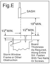
1. Check window opening size-- the mounting parts furnished with this air conditioner are made to install in a wooden sill double-hung window. The standard parts are for window dimensions listed above. Open sash to a minimum of 19 inches(483mm). See Fig.D. 2.Check condition of window-- all wood parts
