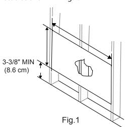
Carefully measure and cut an opening with the following dimensions depending on your model. See Fig.1 and Fig.2.
