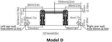
**NOTE:** When the gas side connective pipe is  $\Phi$  16mm(5/8in) or more, the wall hole should be 90mm(3.54in).
