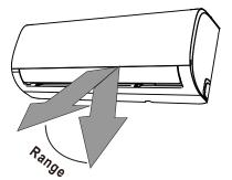
**NOTE:** Do not move louver by hand. This will cause the louver to become out of sync. If this occurs, turn off the unit and unplug it for a few seconds, then restart the unit. This will reset the louver.
