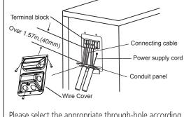
Please select the appropriate through-hole according to the diameter of the wire.
