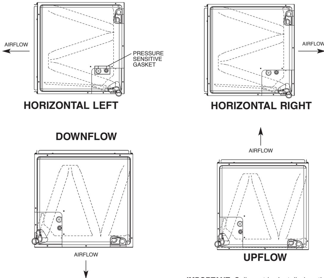
**IMPORTANT:** Coil must be installed on the supply airflow side of a gas or oil furnace.
