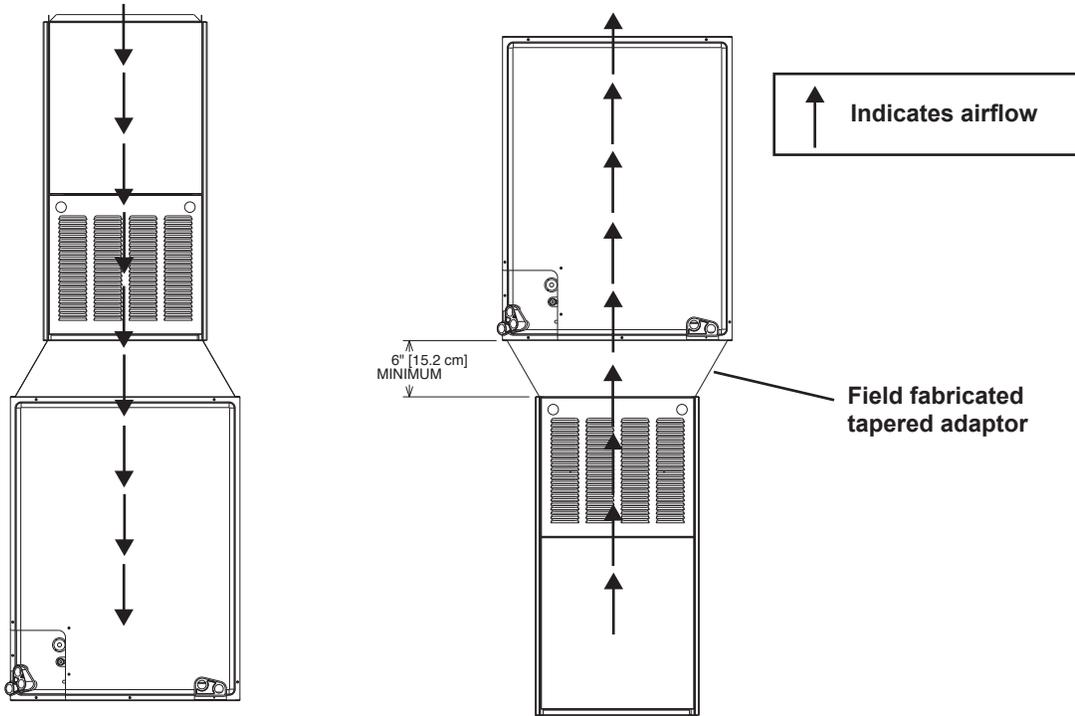
Figure 4: Installation of coil matched with a furnace of smaller size
