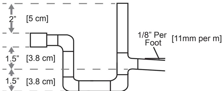
**UNIT MUST BE LEVEL OR SLIGHTLY PITCHED TOWARD DRAIN CONNECTION**
