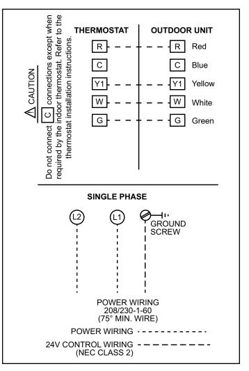
**Figure 5. Typical Wiring Connections**
