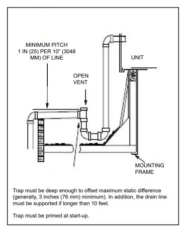
Figure 2. Typical Condensate Drain Connection
