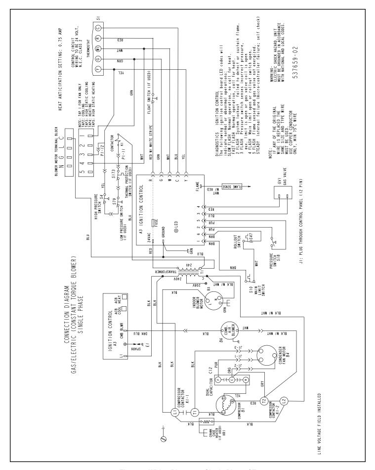
Figure 7. Wiring Diagram - Single Phase CT
