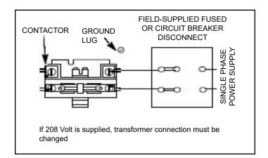
Figure 4. 208/230 Line Voltage Wiring
