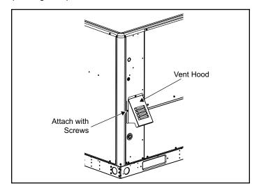
Figure 1. Installing the Vent Cover
