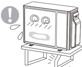
If it is damaged, it may lead to the unit falling and cause injury and damage.
