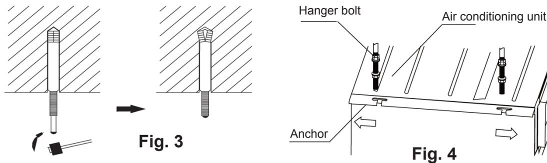
Install the hanger on the indoor unit, as shown in Fig. 4.
