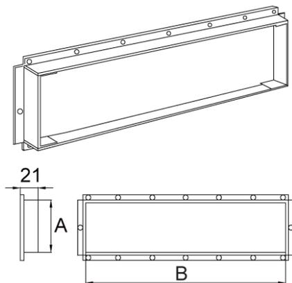
**Fig. 9 Air Supply Outlet**
