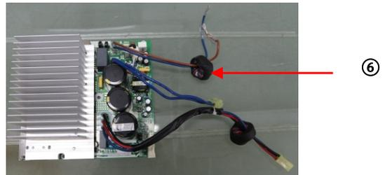
16) Disconnect the connectors and wires connected from PCB and other parts.
