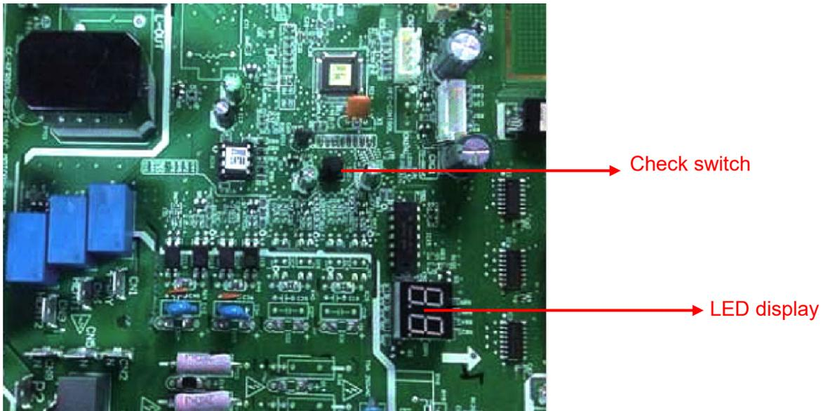
**7.4.2.17 Communication malfunction between adapter board and outdoor main control board (ODU Ed)**
