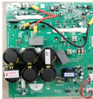
CN8: Discharge temperature sensor (2p, white)
