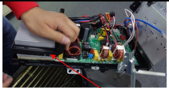
7) Disconnect the connectors and wires connected from PCB and other parts.
