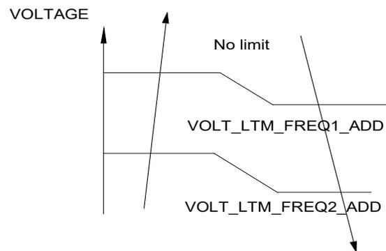
Note: If low voltage protection triggers and voltage is not restored to normal within 3 minutes, the protection remains active even after a machine restart.
