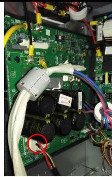
3) Disconnect following 8 pieces of connection wires and connectors between IPM and other parts.
