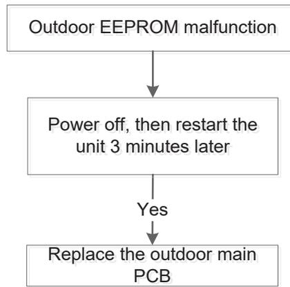
EEPROM: a type of read-only memory. The contents can be erased and reprogrammed using a pulsed voltage.
