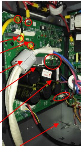
4) Remove the fixing screws then remove the IPM board.
