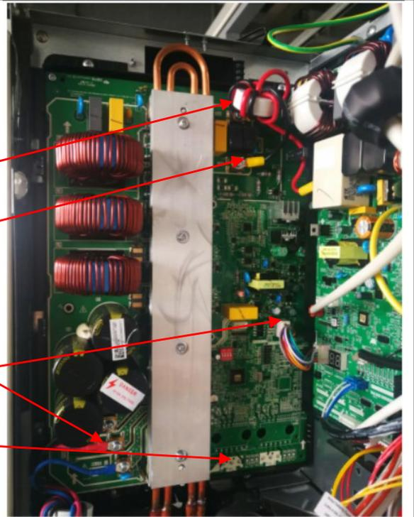
4) Remove the 4 screws and unfix the 4 hooks and then remove the IPM module board.
