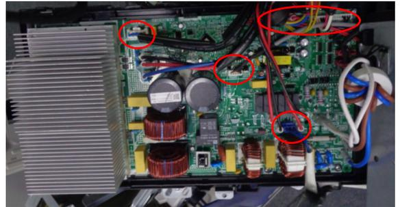
8) Disconnect the grounding wire (yellow - green) after removing the big handle and the right-rear panel.
