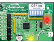
If the **Yellow** LED is off, verify power to the Qwik**Swap**<sup>®</sup> board. If the **RED** LED is off or flashing, there is a communication error.
