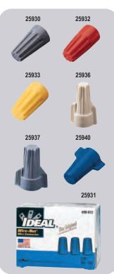
Wing Nut® wire connectors were first introduced by IDEAL in 1958 and remain the most comfortable, easy to use connector on the market. The wings act as a built in wrench to provide extra leverage for secure connections...every time. Wing Nut® wire connectors handle a wide range of branch circuit and fixture wiring requirements. Just three color coded models handle UL listed wire combinations from (2) No. 18's to (1) No. 6 with (2) No. 8's, solid or stranded wire.
