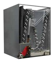
Cased coils are ideal for dual fuel add-on applications. Fully insulated cabinets come with dual right and left hand condensate drain connections. Fully insulated cabinet includes corrosion-proof drain pan, and all aluminum evaporator coil. Equipped with TXV. AHRI certified when matched with HZS split units.
