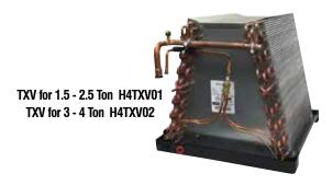
Rifled copper tubing, enhanced aluminum fins. Immersion-tested at 500 psi, then nitrogen-pressurized and sealed. Left-hand refrigerant and plumbing connections. Externally mounted flowrater body with Schrader valve. Heavy duty plastic drain pans on all models. AHRI certifiable with certain brands of A/C and heat pump systems. UL listed for use with both R-22 and R-410a when proper metering device is used.
