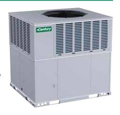
13.4 SEER2, 24 – 60 kbtuh, aluminized steel tubular heat exchanger, horizontal or downflow application, max width of 47" fits in small, standard, and long truck beds. Rugged full perimeter base rails with cornerhoist points and standard forklift slots. Can be rooftop or slab mounted, slide out blower motor for ease of maintenance. RGP: Propane convertible (LP kit included). RHP: Optional field install heat kits available.
