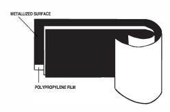
sheets of polypropylene film onto which is "sprayed", or metallized, a thin layer of metal. Two metallized films are then wound together very tightly to form the capacitor. The resulting roll is very hard and cannot be squeezed into a traditional oval shape.
