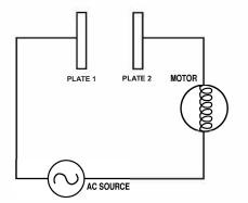
Now let's connect our simple capacitor to a source of AC current and in series with the windings of an electric motor. Since AC current alternates, first one plate, then the other would be charged and discharged in turn.
